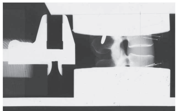
Fig. 1. Radiograph of a vertebral specimen embedded in two metal cups containing dental plaster. Pins inserted into the vertebrae were used to detect vertebral movements.
